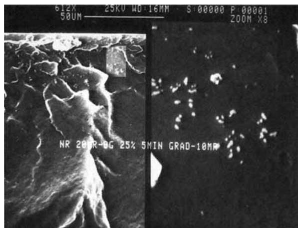
Figure 15 SEM photograph of fractured cross-section of the NBR/bis-GMA asymmetric system. Top of photograph is the surface by which bis-GMA penetrated.
